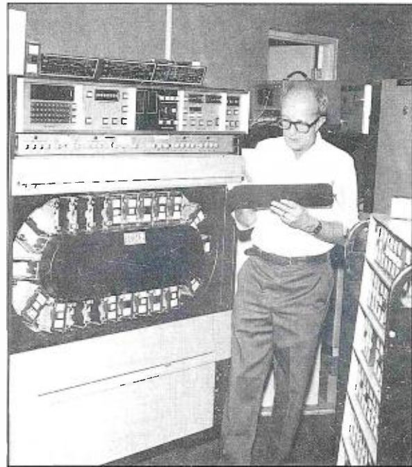
Two TCR-100A "cart" machines handle commercial blocks—about 600 air functions daily.
